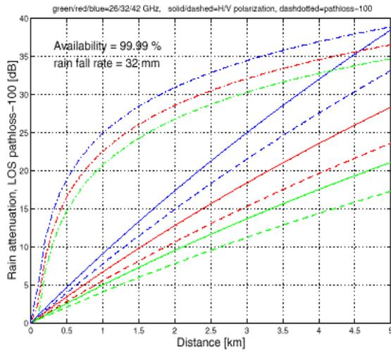
Figure 5. Rain and Path loss for different micro-wave frequencies
