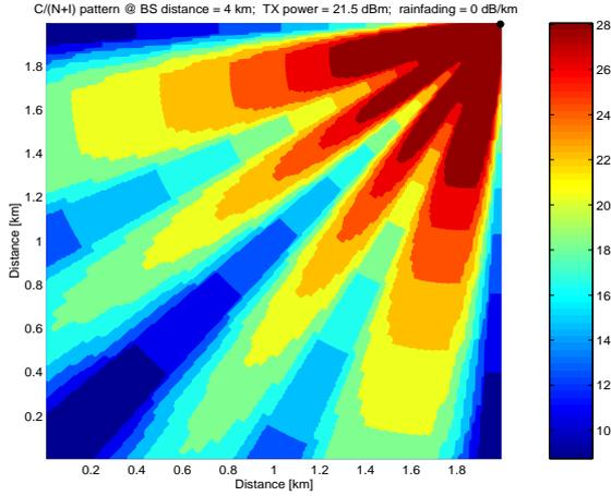
Figure 4. C/(N+I) Distribution in a worst sector of a Rectangular 5x5 Multi-cell Configuration
