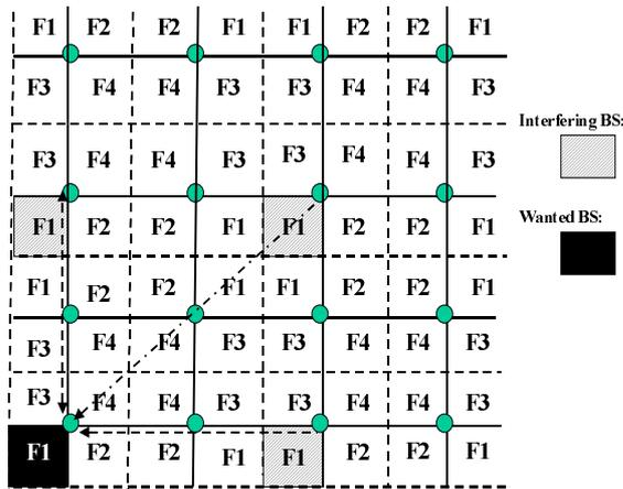
Figure 2. A Rectangular 4x4 Multi-cell Configuration with 4 Frequencies
