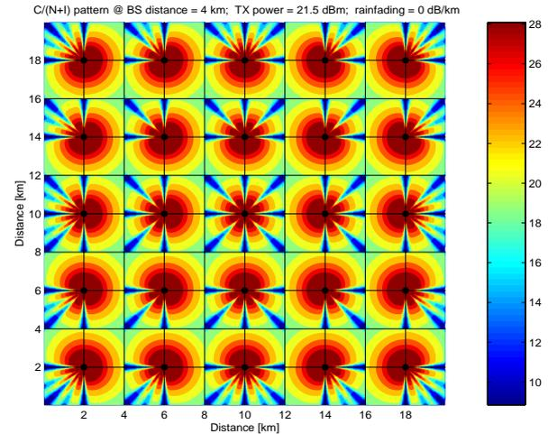
Figure 3.  $C/(N+I)$  Distribution in a Rectangular 5x5 Multi-cell Configuration
