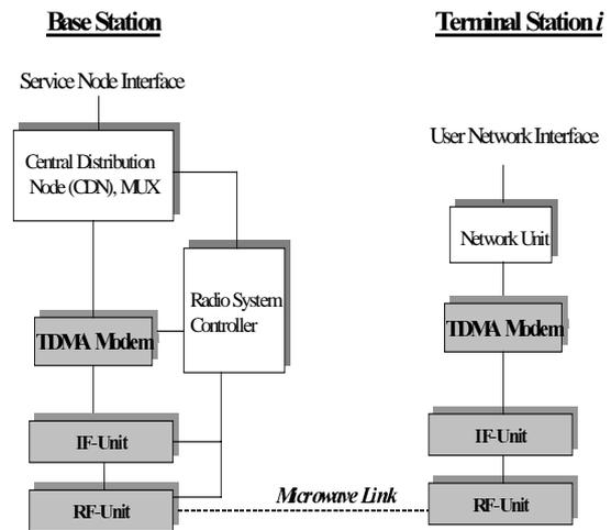
Figure 1. Digital microwave PMP-transmission system based on TDM/TDMA
