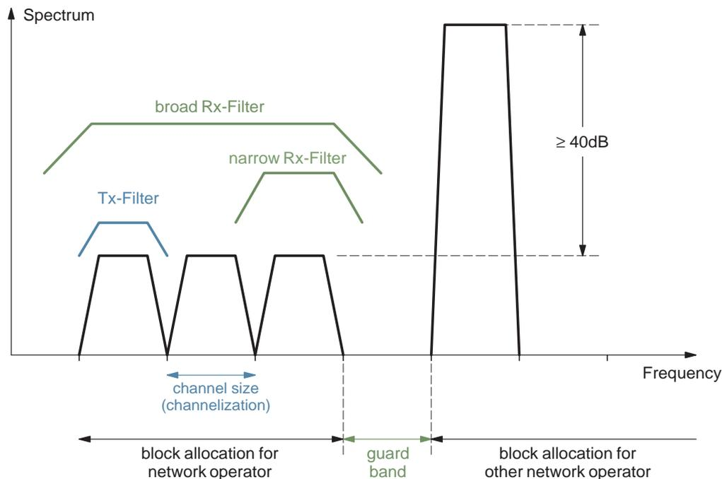
**Figure 1: Frequency allocation for two adjacent network operators (with independent cell planning, assuming worst-case power ratio)**
